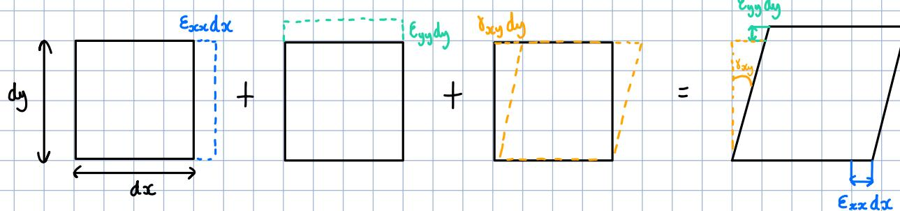
Plane Strain: deformations limited to XY Plane
